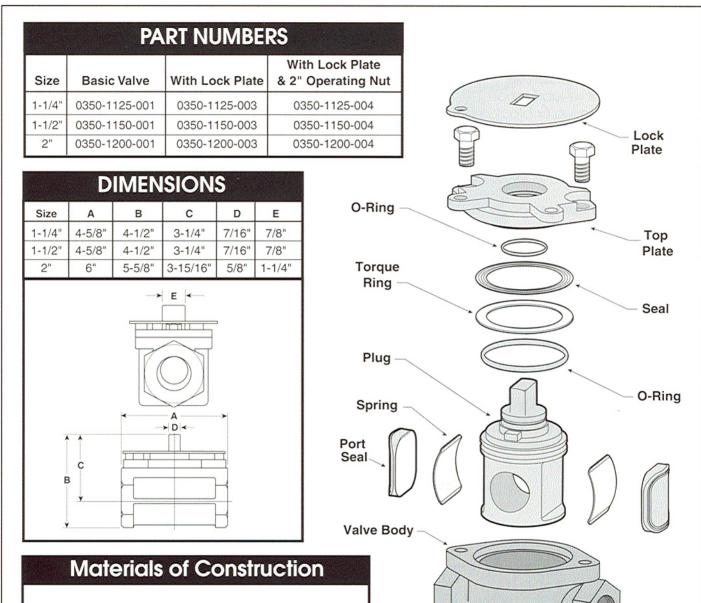
Body & Top Plate: Ductile Iron, ASTM A 536 GR 65-45-12
